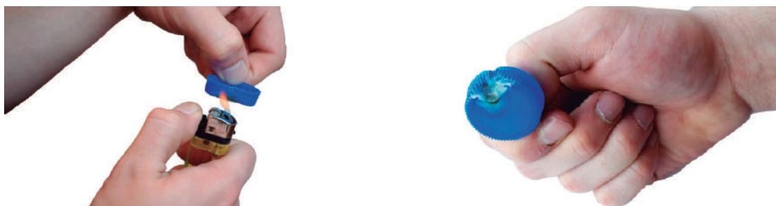
Figure 70 HDPE in contact with the flame
