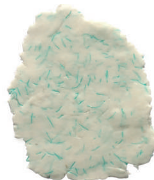
Figure 62 Sample 2 (silicone, potato starch and shredded fishing net)
