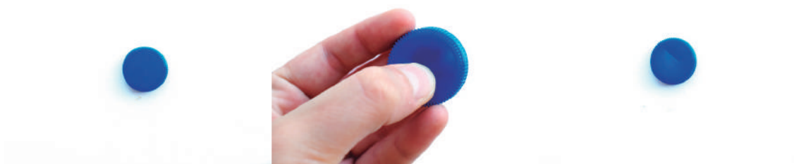
Figure 72 Scratching test on HDPE lid with the nail (before, during and after)
