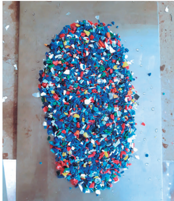
Figure 74 The shredded HDPE on top of the stainless-steel plate
