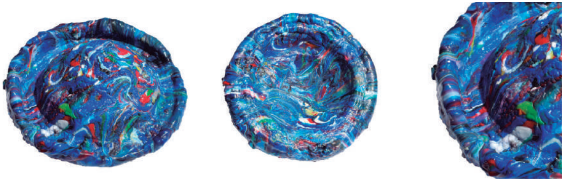
Figure 91 Plaster casting moulding prototype: 1st experience - mould coated with cling wrap
