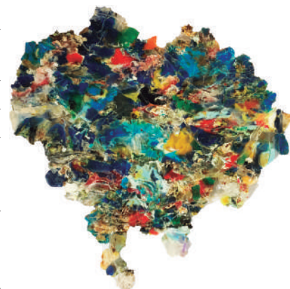
Figure 75 Sample 1 (HDPE bottle caps and fishing net)
