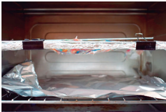
Figure 105 HDPE sheet deformation in the furnace
