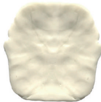
Figure 61 Sample 1 (silicone and potato starch)
