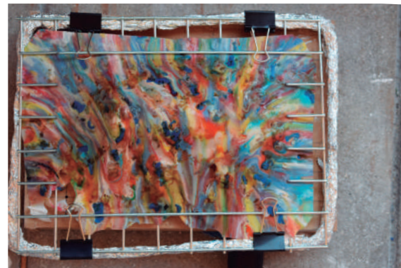
Figure 107 HDPE sheet on top of the plaster mould
