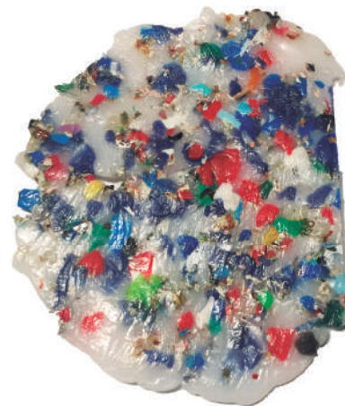
Figure 80 Sample 6 (Raw and recycled HDPE)
