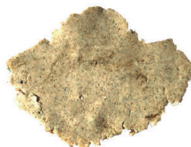
Figure 65 Sample 5 (silicone, potato starch and sand)
