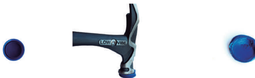
Figure 71 Smashing one HDPE lid with the hammer (before, during and after)
