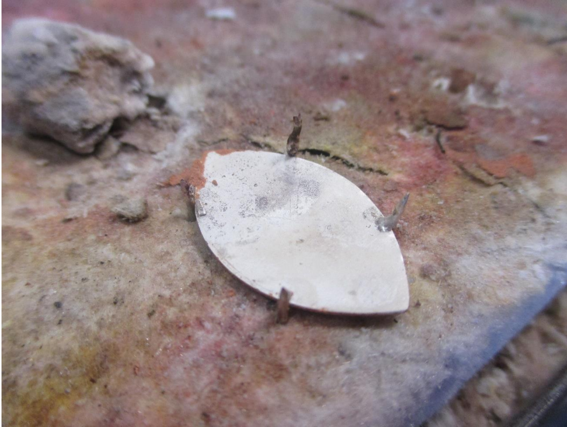
Figure 52. Welding the navete-shaped piece.
