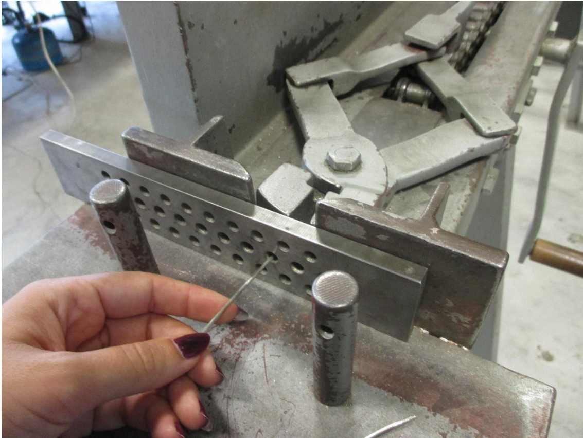
Figure 45. Pulling the metal plate to make it cylindrical.
