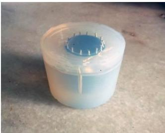
The mixture was then poured in to the mould.
