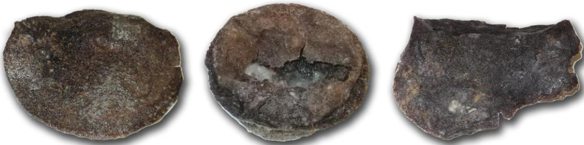
**Figure 31 - Starch experiments showing signs of moisture with the appearance of mold.**
