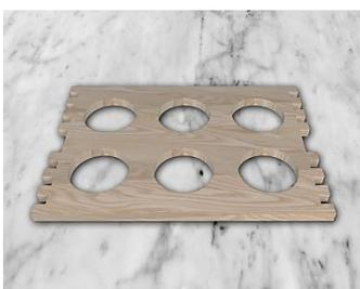
For the laser cut, the CAD part was converted to DWG (2D) and from that, an operative programmed a laser cutting machine to cut a wooden board with the aid of software. The machine used for this task is from Hanma Laser, as is the software that programmes it.
