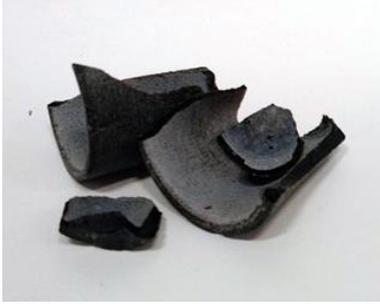
**Figure 37 - Sample after being machine washed.**
