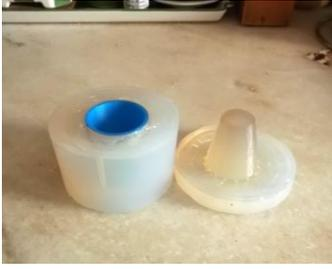
The silicone used for the mould was 950 VTX, provided by SLM and the catalyst proportion was 10%. The curing time was 24 hours as usual with this type of resin.
