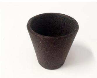
After 10 to 15 minutes, which was normally the time for it to dry, the result could be taken out of the mould.
