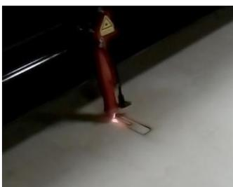
For the wooden part, the chosen method was by laser cutting, as it was the fastest and most precise method.
