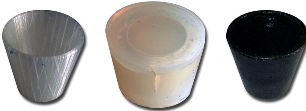
Figure 39 - Creation of a second, bigger mould for the cups.
