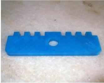
For the base legs/handles, again a 3D printed piece was produced.
