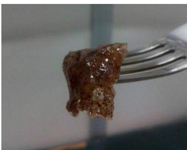
**Figure 32 - Deteriorated coffee/starch mixture after being submerged in cold water.**
