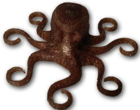
**Figure 20 - 3D Printer, property of FEUP (left). 3D printed octopus using 3Dom coffee filament (right).**
