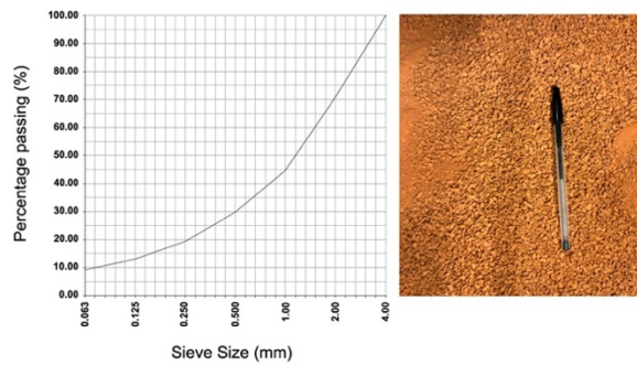
Fig. 1. Granulometric curve of recycled brick sand (left), and image of the same sand (right).
